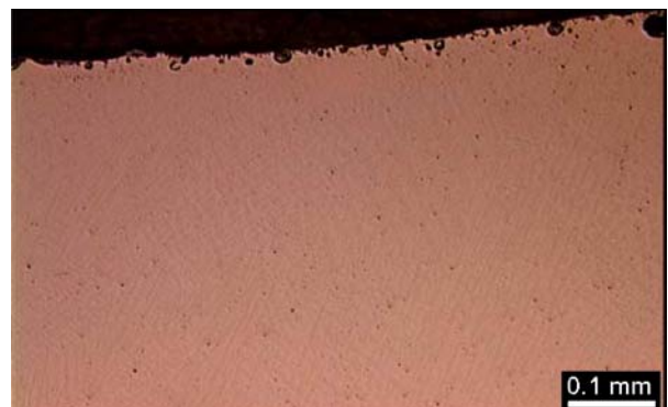
Figure 6 Gas bubbles and shrinkage porosity on the Cu-30Ni clad.
