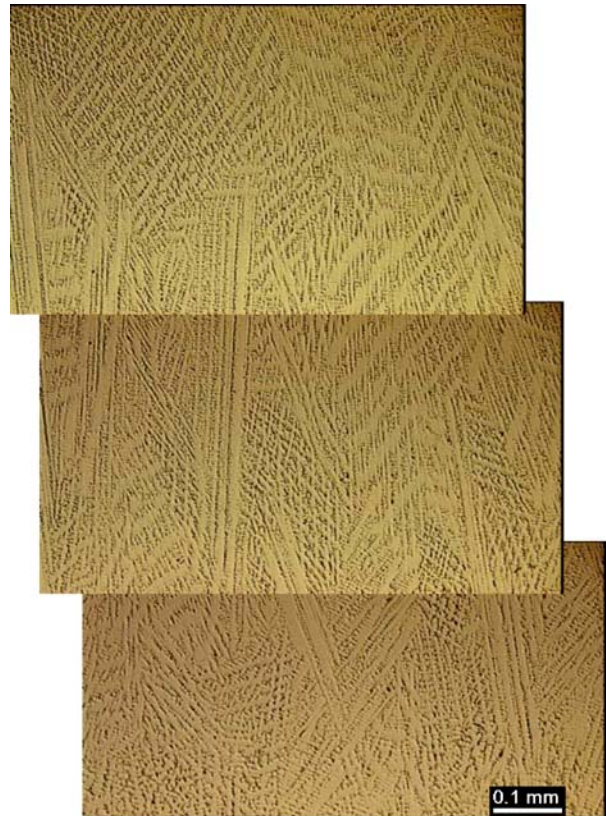
Figure 2 Dendritic solidification of Cu-30Ni clad material and melted substrate with strong (1 0 0) texture.
